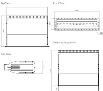
FIBER-REX offers an innovative, robust, high density 3U Chassis. This panel has been designed to accept up to 14 LGX style assemblies. With the ability to use a full array of adapter types offering a flexible solution to the end user, The multifunctional chassis allows the user easy access during installation or re-work without disturbing of the existing cable or fibers.
